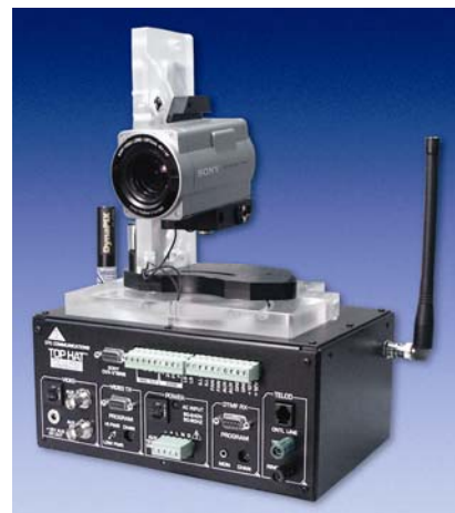
Figure 9. PTZ Camera TX
